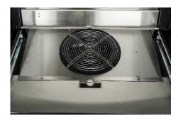
With the base tray pulled out, sweep out, or use a vacuum cleaner, to remove any debris from the base cavity.
