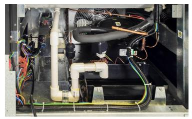
The compressor, condenser fan and condensate disposal system are mounted in the base of the cabinet, behind the condenser radiator.
