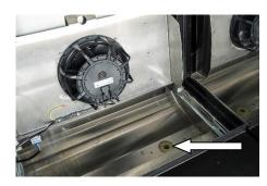
After removing the fixing screws, the fan deck can be lifted and unplugged from the cabinet for thorough cleaning.
