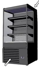
Use a vacuum cleaner to remove dust and fluff from the ventilation louvers on the front and top of the cabinet.
