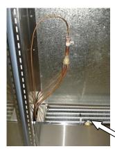
With the back plates removed, the cooling coil is exposed. No cleaning is normally required, but if there is any debris visible, carefully remove it with a vacuum cleaner.
