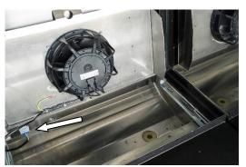
The fan deck is connected to the cabinet with a plug and socket, and can be withdrawn to replace a faulty fan, after removing the fixing screws.
