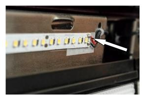
The LED strip is self-adhesive, with soldered connections.
