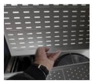
The evaporator coil and temperature probes are accessed by removing the inside back panel of the cabinet.
